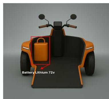
Figure 2. A view of 72 V lithium-ion battery pack from entry side
