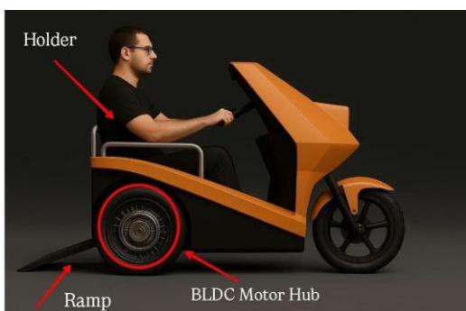
Figure 1. Vehicle side view showing ramp, holder, and hub motor
