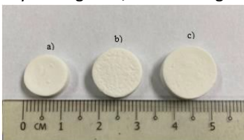
Impregnation of Labisia pumila into hybrid alginate/starch aerogel
