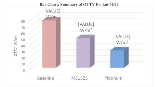
The bar chart above demonstrates that improving glass U-value can reduce 37% of OTTV (comparison between Baseline and MS1525). While, improving glass U-value and WWR can reduce 63% of OTTV (comparison between Baseline and Platinum), and 41% of OTTV (comparison between MS1525 and Platinum). Source: Zainonabidin (2015)
