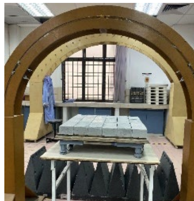
Fig. 3. NRL Free Space Arch Measuring setup.
