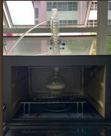
Microwave-assisted extraction set-up
