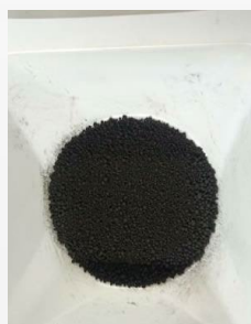
Biochar of Used Mashaf obtained under Microwave Pyrolysis
