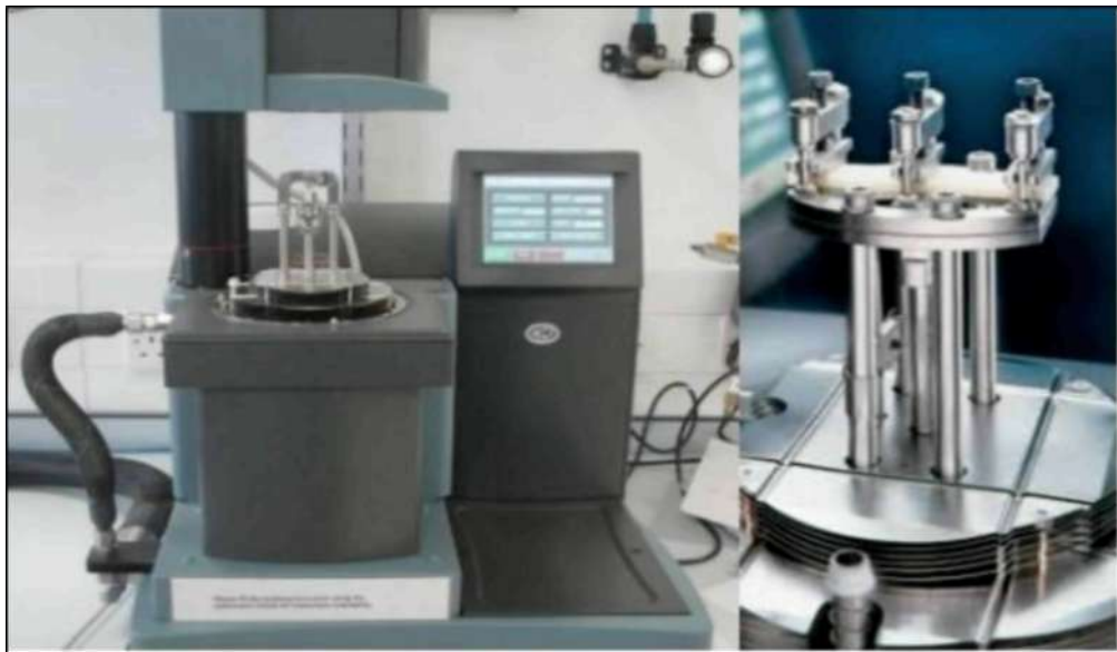
Figure 3. 12 Dual Cantilever Mode Used for Dynamic Mechanical Analysis (DMA)
