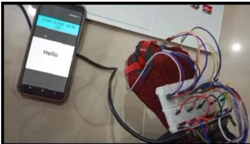
Figure 2: The prototype model of Sign Glove with IoT
