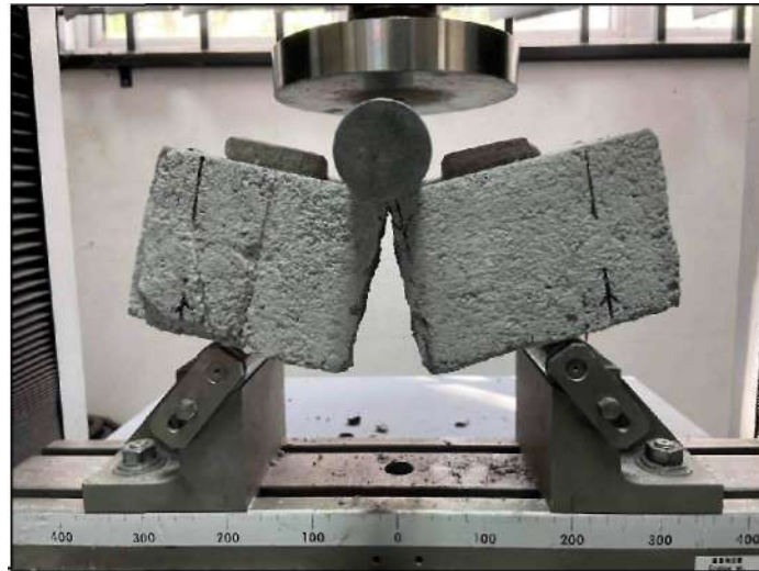
Figure 4.64 The Split Crack of Single Inclined Connection Interlocking Block (SICIB)
