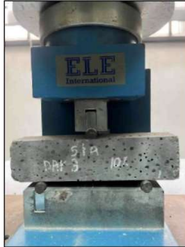
Figure 4.25 Sample 3 Days After Flexural Test
