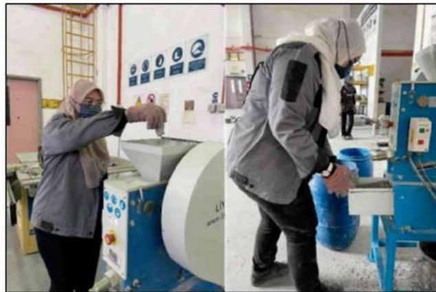
Figure 3.13 Crushing the Concrete Cube to the Small Particle using Jaw Crusher
