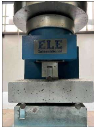
Figure 4.31 Sample 56 Days After Flexural Test
