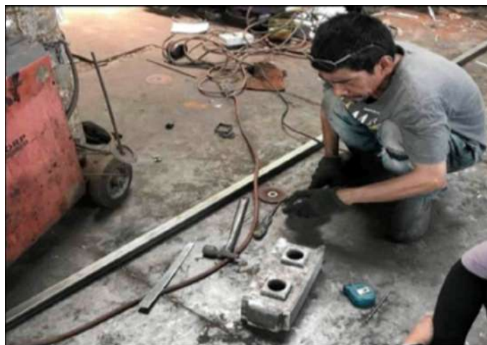
Figure 3.36 Steel Mould Preparation formwork for interlocking block design
