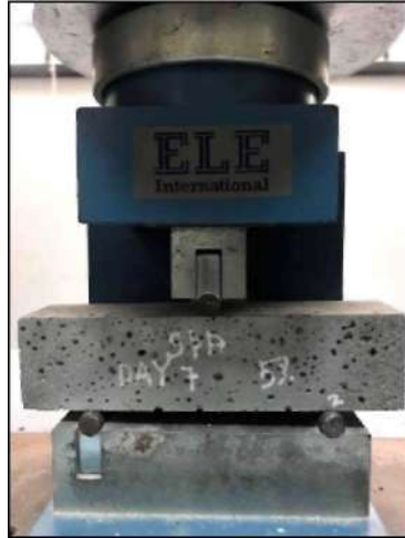
Figure 4.27 Sample 7 Days After Flexural Test
