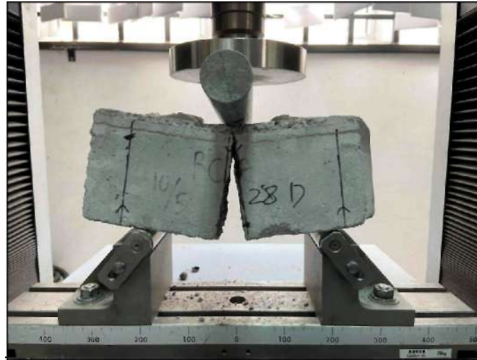
Figure 4.65 The Split Crack of Dual Tongue Inclined Interlocking Block (DTIIB)
