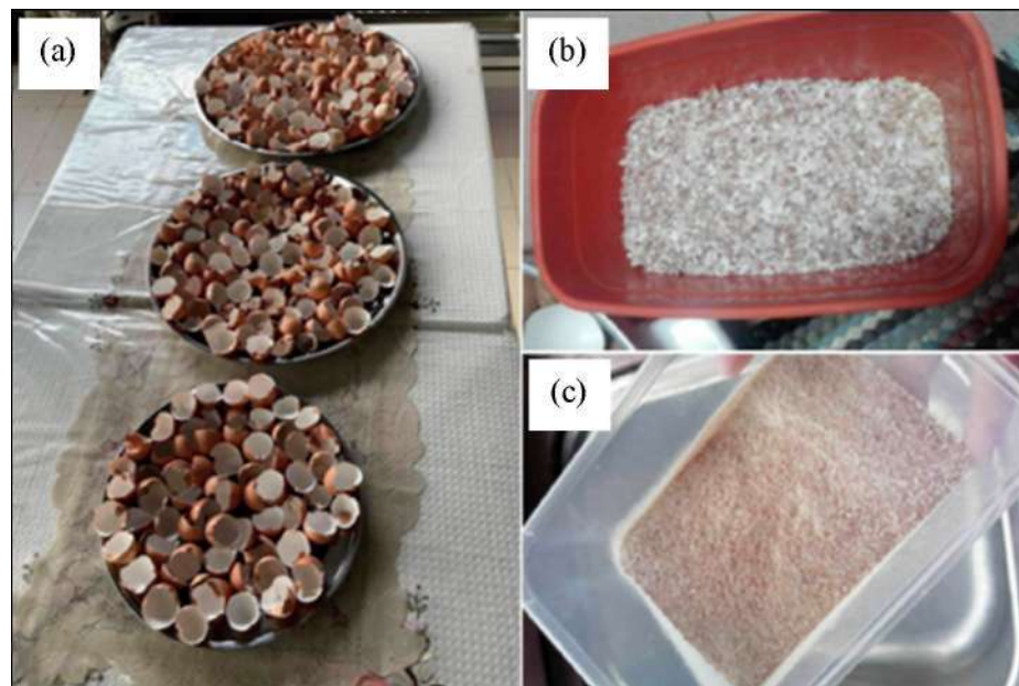
Figure 3.5 Changes State of Eggshell: (a) Washed Fresh Eggshell; (b) First Condition After First Session of Grind; and (c) Second Condition After First Session of Blend
