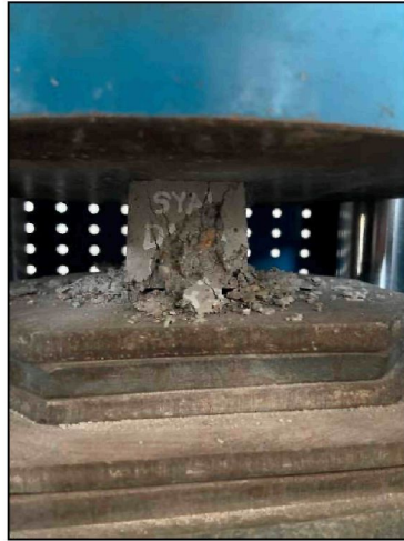
Figure 4.19 Sample 56 Days After Compression Test
