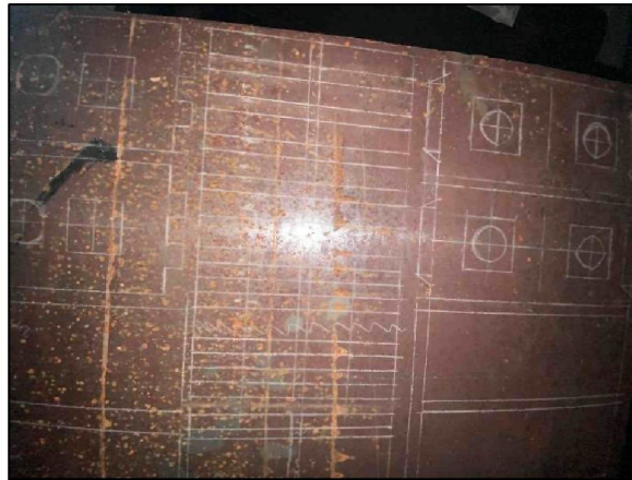
Figure 3.35 Steel Mould for Single Inclined Connection Interlocking Block (SICIB) and Dual Tongue Inclined Interlocking Block (DTIIB)
