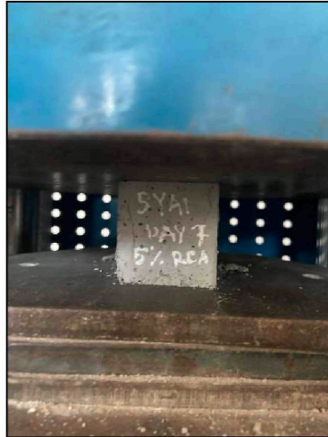
Figure 4.15 Sample 7 Days After Compression Test
