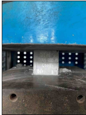
Figure 4.11 Sample OPCNA After Compression Test
