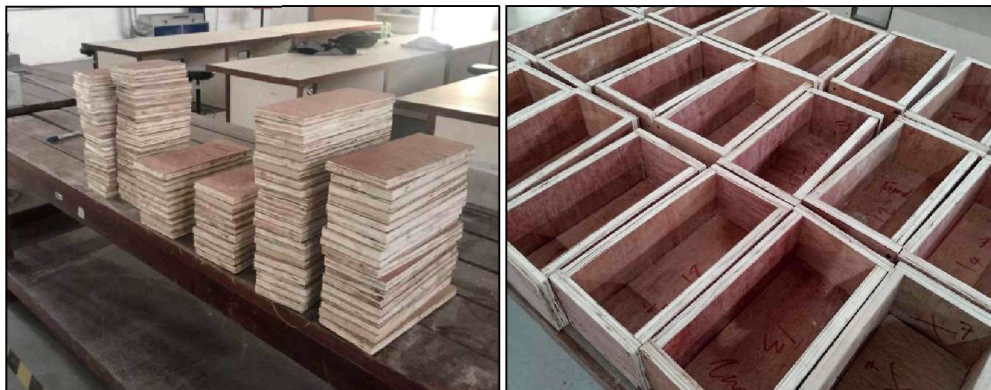
Figure 3.34 Plywood Mould for Solid Interlocking Block (SIB)
