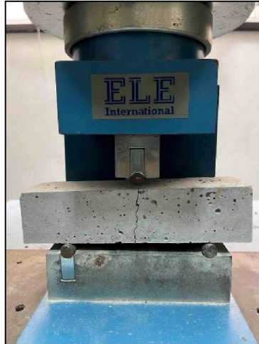
Figure 4.23 Sample 56 Days OPCNA After Flexural Test
