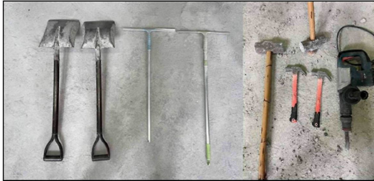
Figure 3.12 Tools Used for Crushing and Handling the RCA at First Stage
