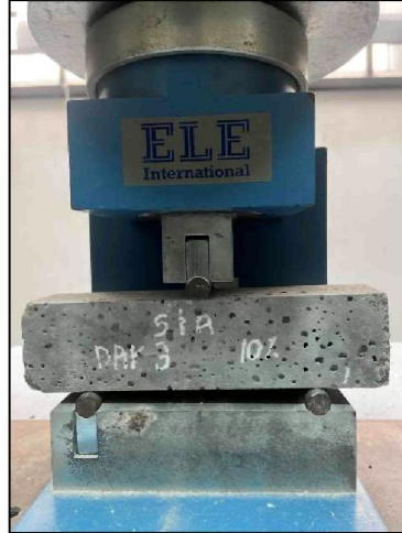
Figure 4.25 Sample 3 Days After Flexural Test
