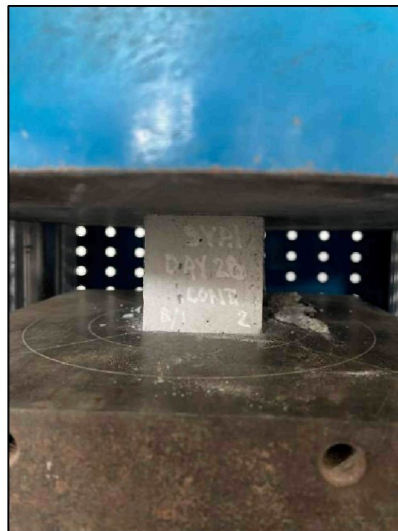
Figure 3.25 Cube (50 mm X 50 mm X 50 mm) Set Up
