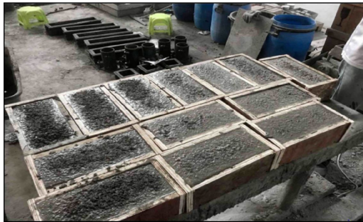
Figure 3.39 Condition of Mixture After Vibrated Using Vibrator Plate Machine
