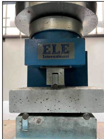
Figure 4.31 Sample 56 Days After Flexural Test
