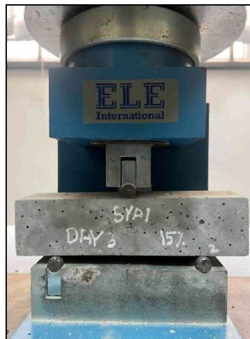
Figure 3.27 Prism Set Up used suitable Three-Point Loading for 160 mm X 40 mm X 40 mm Prism
