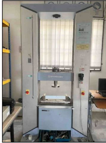
Figure 3.26 Universal Testing Machine 100 kN
