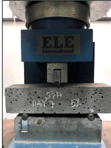
Figure 4.27 Sample 7 Days After Flexural Test
