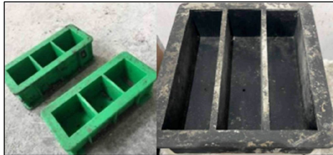
Figure 3.19 Plastic Mould for Cube and Prism Samples
