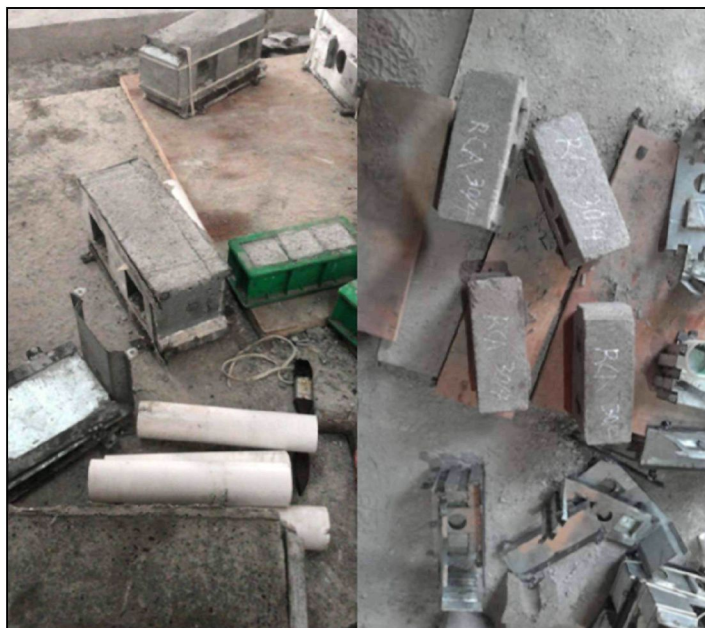
Figure 3.40 Filled Mould Dried for 24 Hours
