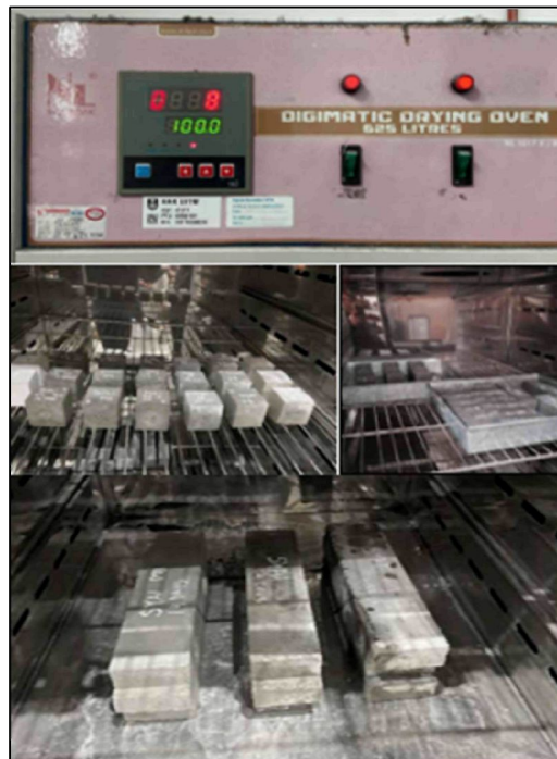
Figure 3.23 Sample in Oven for 2 hours with 100°C
