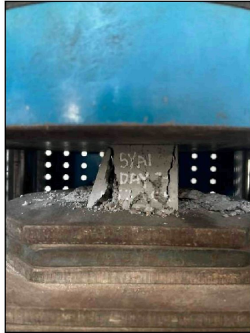
Figure 4.17 Sample 28 Days After Compression Test
