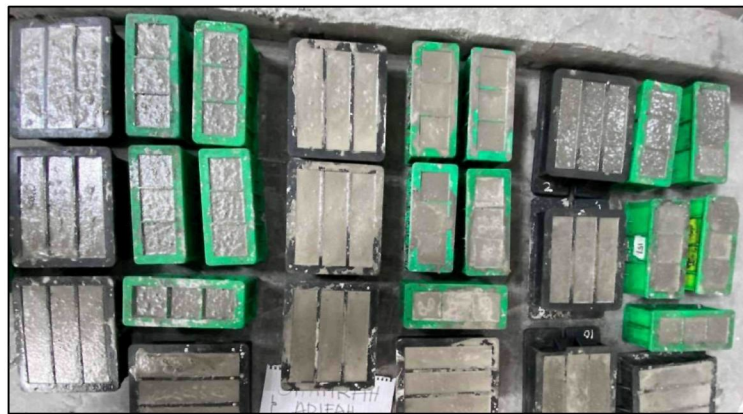
Figure 3.20 Casting of Cube and Prism Samples
