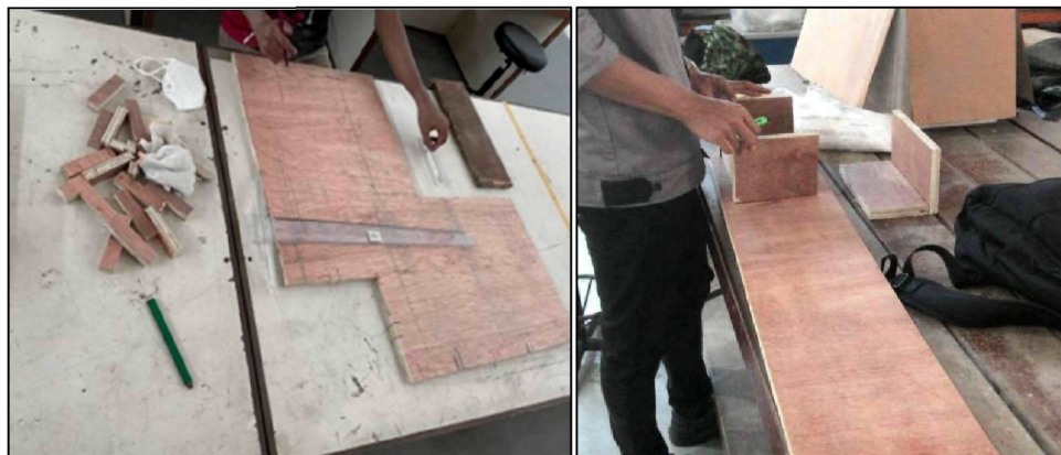
Figure 3.33 Sketch on Plywood Mould for Solid Interlocking Block (SIB)
