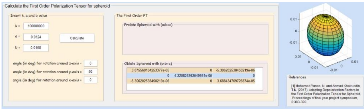
Figure 5: The interface when using the GUI with inputs conductivity, k = 100000000 , semi axes, a = 0.0124 , and b = 0.0156 with \theta = 50^\circ .
