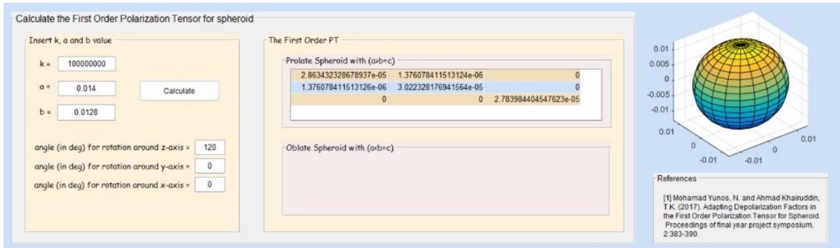
Figure 4: The interface when using the GUI with inputs conductivity, k = 100000000 , semi axes, a = 0.014 , and b = 0.0128 with \theta = 120^\circ .
