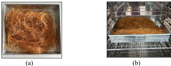
Fig. 1. Preparation of coconut fibre (a) Raw coconut fibre after wash; (b) Drying process using oven
