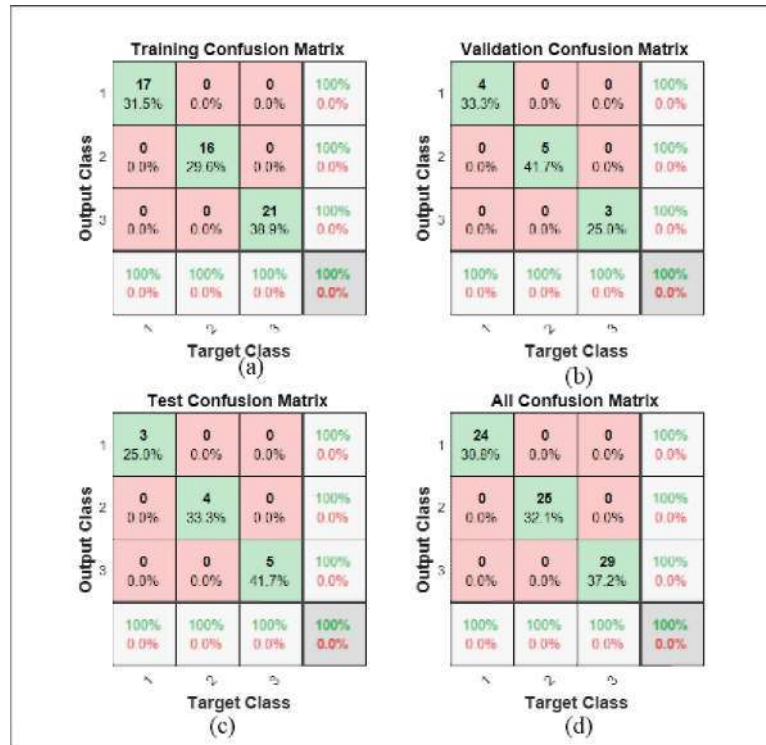
Figure 4.24 Confusion Matrices for L-band Slot Size Classification Using the LM Algorithm: (a) Training, (b) Validation, (c) Testing, (d) Overall
