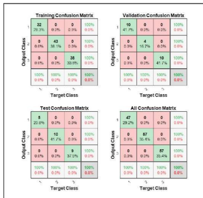
Figure 4.35 Confusion Matrices for S-band Slot Size Classification Using the SCG Algorithm: (a) Training, (b) Validation, (c) Testing, (d) Overall
