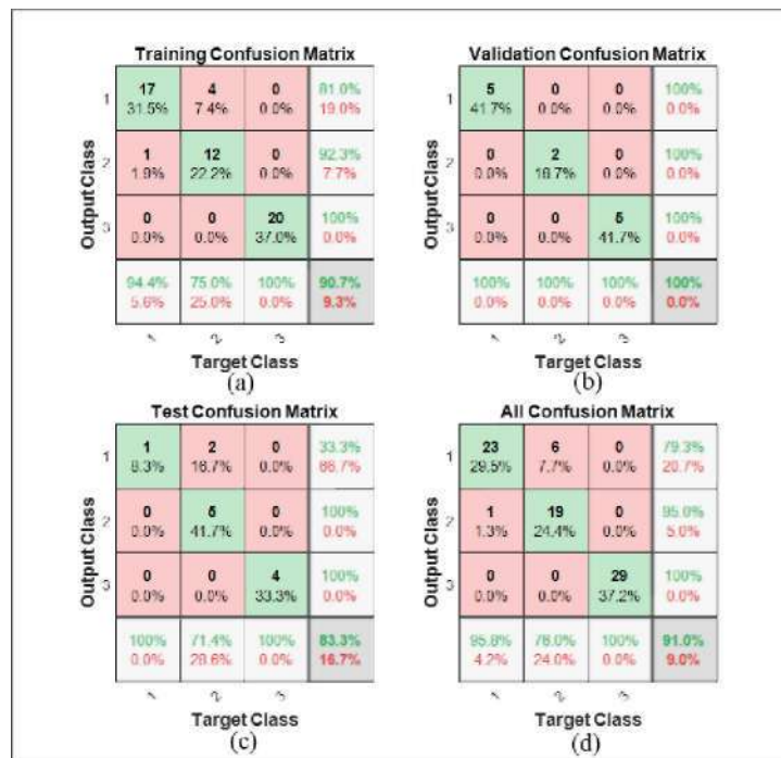
Figure 4.28 Confusion Matrices for L-band Slot Size Classification Using the SCG Algorithm: (a) Training, (b) Validation, (c) Testing, (d) Overall
