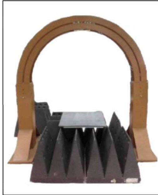
Figure 3.2 The Free Space Arch Measurement Set Up [22]
