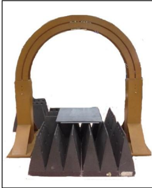
Figure 3.2 The Free Space Arch Measurement Set Up [22]
