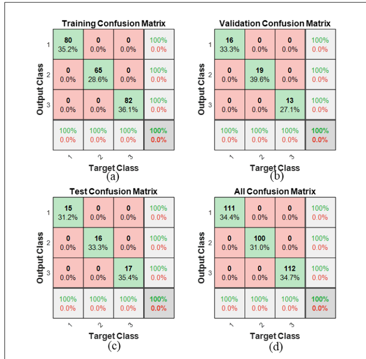
Figure 4.38 Confusion Matrices for C-band Slot Size Classification Using the LM Algorithm: (a) Training, (b) Validation, (c) Testing, (d) Overall
