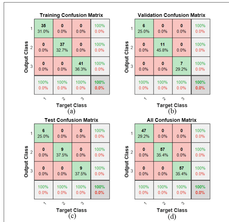
Figure 4.31 Confusion Matrices for S-band Slot Size Classification Using the LM Algorithm: (a) Training, (b) Validation, (c) Testing, (d) Overall
