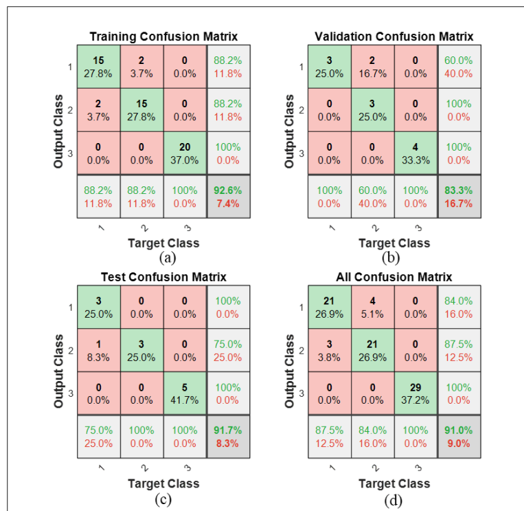
Figure 4.26 Confusion Matrices for L-band Slot Size Classification Using the RBP Algorithm: (a) Training, (b) Validation, (c) Testing, (d) Overall
