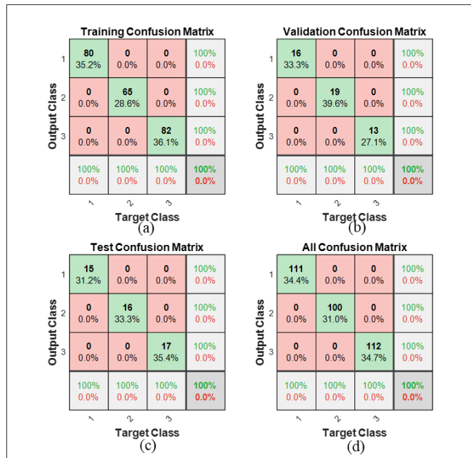
Figure 4.42 Confusion Matrices For C-band Slot Size Classification Using the SCG Algorithm: (a) Training, (b) Validation, (c) Testing, (d) Overall
