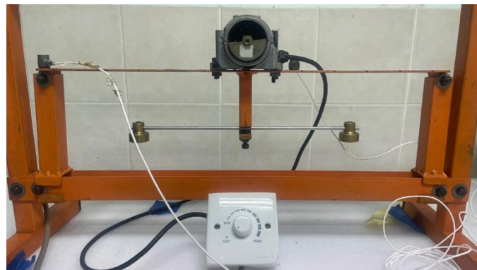
Figure 2: The TDVA attachment of the unbalanced motor-beam system.
