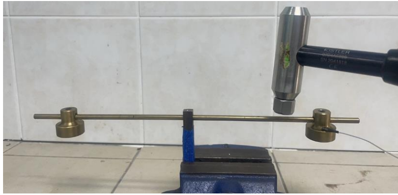
Figure 2: Impact testing to a mass's beam.
