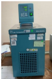
Fig. 2. Refrigerated bath circulator for electrolyte temperature control
