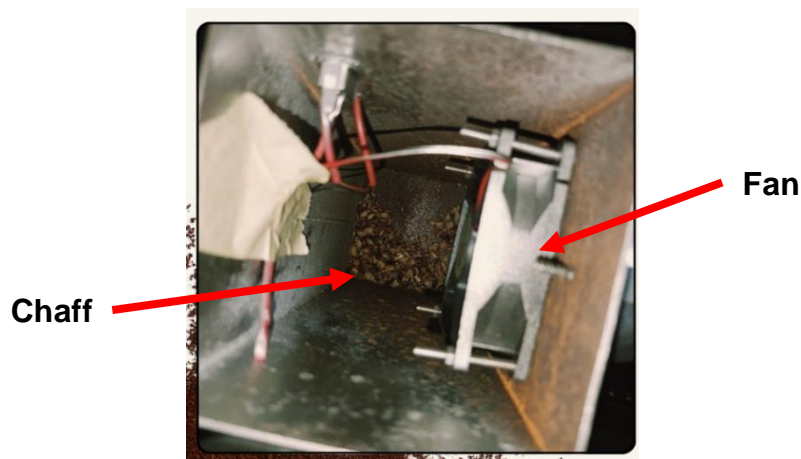
Figure 3: The Internal Layout of Chaff Collector Machine with Chaff Collected
