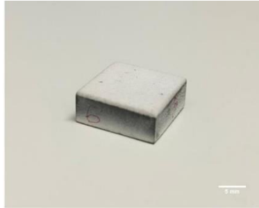
Figure 0.1 Specimen size: 15mm x 15mm x 6mm.
