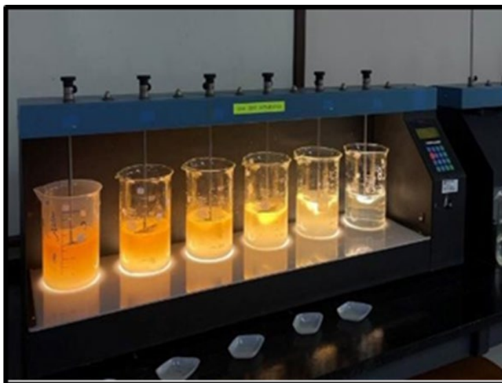
Figure 4. Jar test experiment on the coagulation process.
