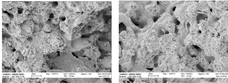
Fig.14 : Fracture morphologies of of (a) PW part sintered at 1210°C, (b) PS part sintered at 1210°C
