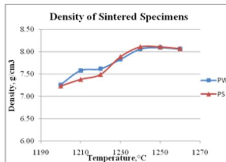
Fig. 11: Effects of sintering temperature on the density of sintered parts.
