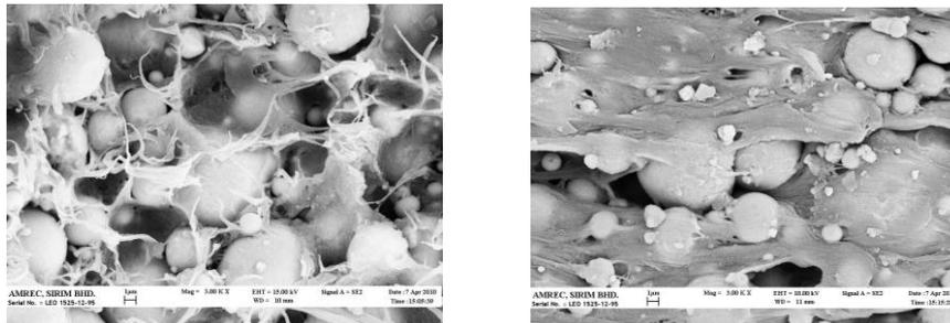
Figure 6. Scanning electron micrograph of (a) fractured surface of the green body (b) surface of the green body.
