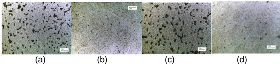
Fig.13 : Microstructure of (a) PW part sintered at 1200°C, (b) PW part sintered at 1250°C, (c) PS part sintered at 1200°C, (d) PS part sintered at 1250°C
