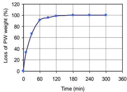
Figure 8. Correlation of binder removal efficiency and debinding time.
