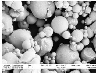
Figure 4. Scanning electron micrograph of commercial M2 HSS powder.
