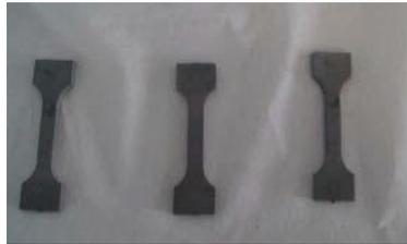
Figure 5: Injection moulded M2 HSS tensile test parts
