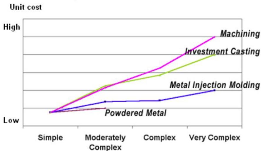
Figure 1.1: Comparison of manufacturing methods as influenced by specimen cost and complexity (SSI Technologies, Inc., 2008)
