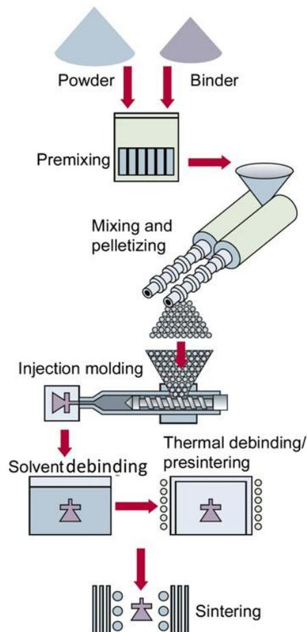
Fig. 2—Schematic of generic metal injection molding processes: feedstock formulation, injection molding, debinding, and sintering: [23] .
