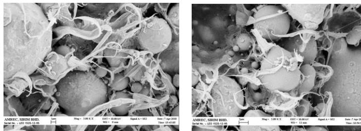
Figure 9: Scanning electron micrograph of fractured surface of (a) leached for 60 minutes (b) leached for 120 minutes
