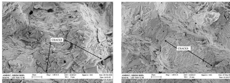
Fig.15 : Fracture morphologies of of (a) PW part sintered at 1260°C, (b) PS part sintered at 1260°C
