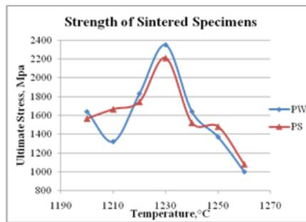
Fig. 10: Effects of sintering temperature on the strength of sintered parts.
