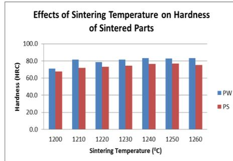
Fig. 12: Effects of sintering temperature on the hardness of sintered parts
