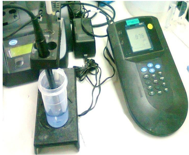
Fig. 1: Traditional pH meter
