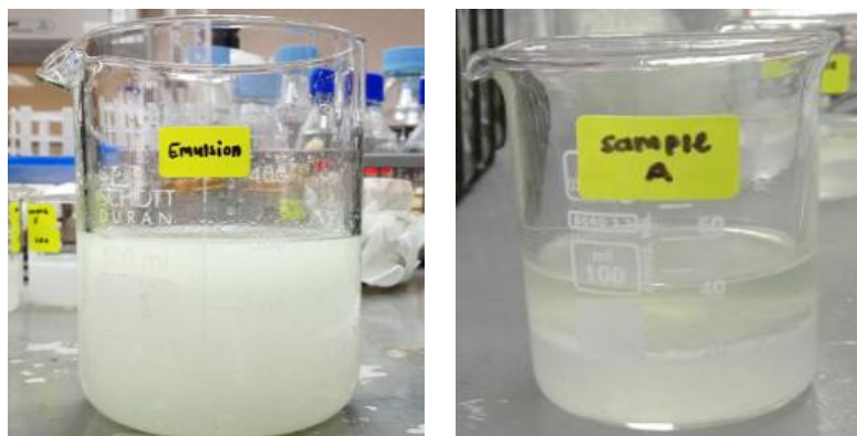
Fig. 1. (left) Preparation of O/W emulsion; (right) O/W emulsified Sample A
