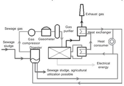
Figure 2: The Field Transformation of Sewage Sludge into Biogas, which in Turn Generates Electrical Energy [7]
