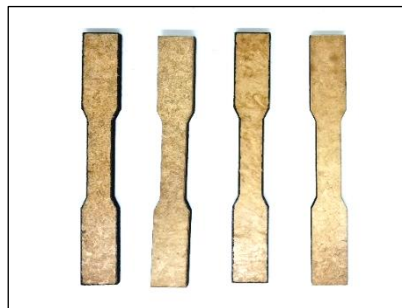
Fig. 5. A tensile test specimen of CM2, CM4, CM6 and CM8 following laser cutting.
