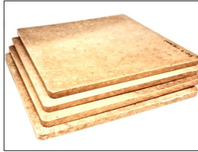
Fig. 4. The composite plate of PALF-TBP following the compression process.
