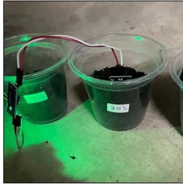
Fig. 5. Moisture sensors were inserted into each soil sample for evaluation of sensor and system performance.
