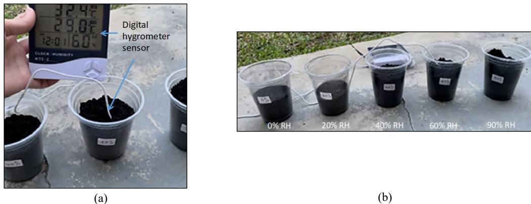
Fig. 4. Soil samples preparation (a) the prepared soil samples were tested with a digital hygrometer sensor to measure the %RH level and (b) soil samples were prepared at 0%, 20%, 40%, 60% and 90% RH conditions.
