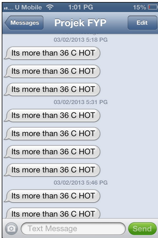
Figure 7: Short message receive from GSM module by using personal mobile phone. SMS are sent once the device detects temperature more than 36°C.
