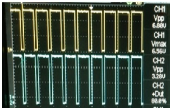
Figure 10: 80% of PWM duty cycle.
