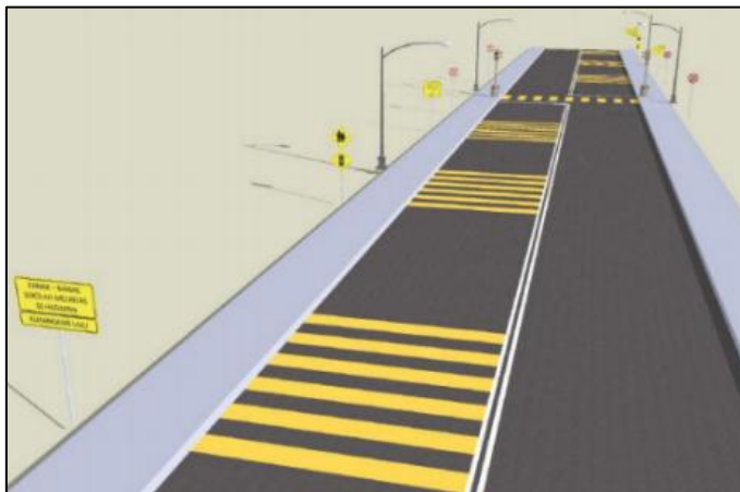
Fig. 6. Sketch of Signalised Pedestrian Crossing at School Zone
