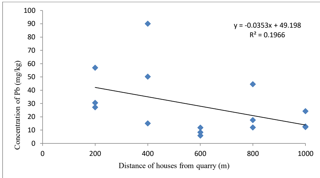
Fig. 9. Concentration of Lead and Distance from The Quarry (m)
