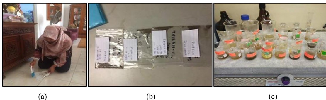
Fig. 2. (a) Collection of the Indoor Dust, (b) Samples of Indoor Dust, (c) Digestion Process
