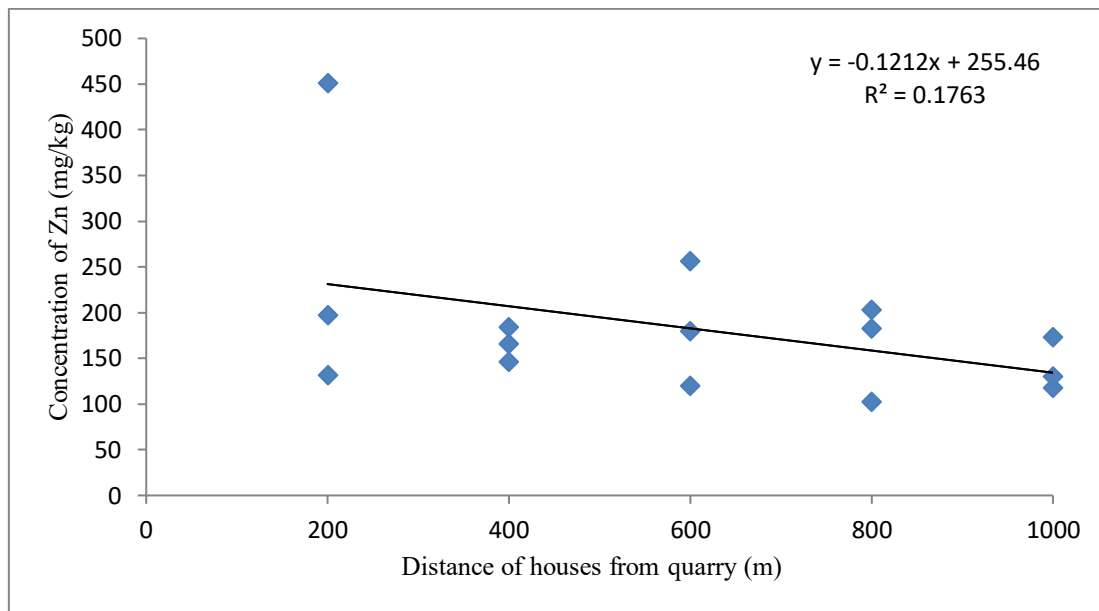
Fig. 10. Concentration of Zinc and Distance from The Quarry (m)
