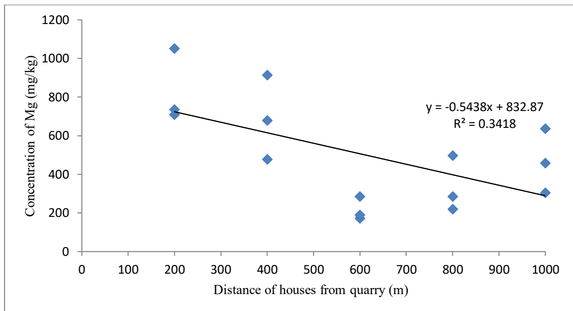
Fig. 6. Concentration of Magnesium and Distance from The Quarry (m)
