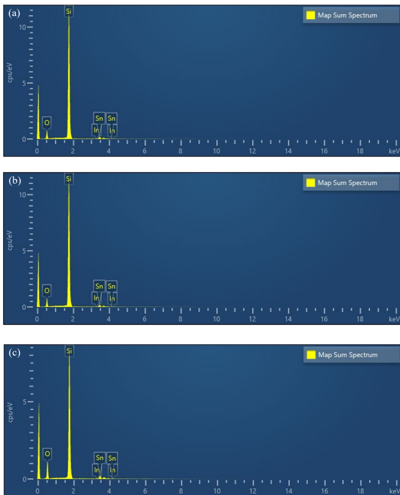
Figure 2: EDX spectrum of ITO thin film at various deposition temperatures (a-c) 1000, 1100 and 1200 °C.
