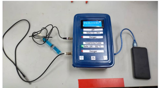
Fig. 8. Complete system of water quality monitoring system with IoT.
