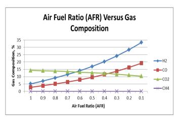
Fig. 9: Graph of Air Fuel Ratio (AFR) versus gas composition
