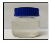
After the raw gas flow through condenser and two filter beds consist of sawdust and activated carbon. Another sample is taken. This is to know the effectiveness of the type of material use as a filter to trap the tar.
