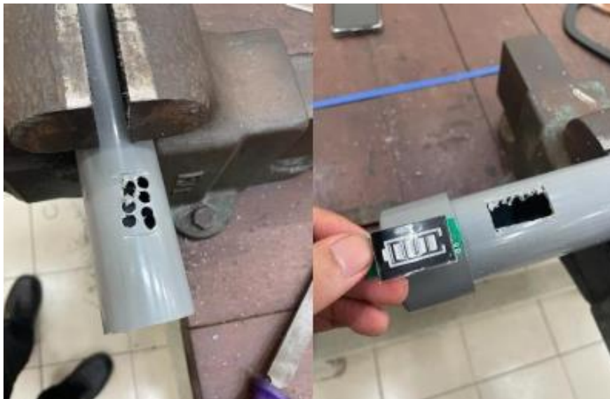
Fig 2: Holes are drilled into the PVC body
