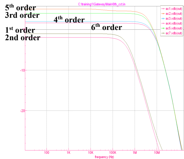
Figure 8. The Butterworth LPF response for different filter's order.
