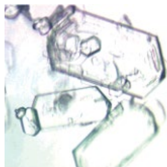
Figure 3.1: Morphology of Aspirin crystal obtains by experimental method [1].
