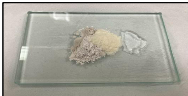
Fig. 2. Mixing of Calcium Sulfate & Chitosan with Distilled Water
