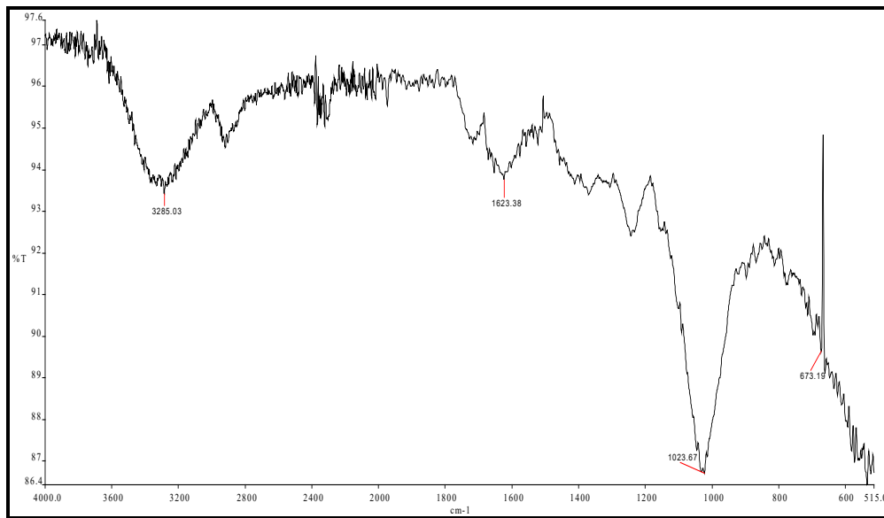
Fig. 5. FTIR spectra of untreated pineapple peels
