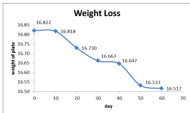
Figure 9: Graph of TPS film weight loss
