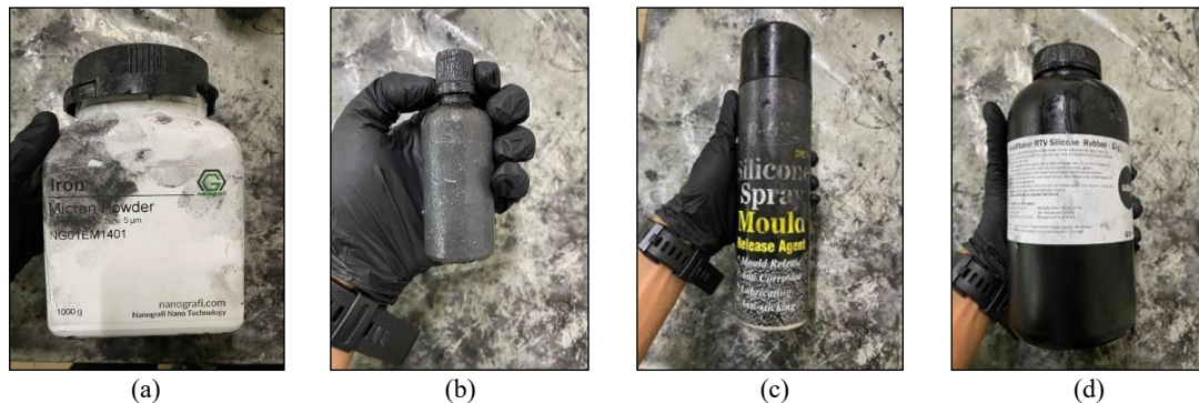
Fig. 1. Material to fabricate MRE (a) carbonyl iron particle (b) hardener (c) silicon spray and (d) RTV silicon rubber.
