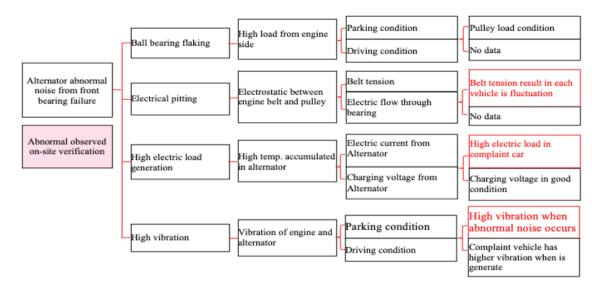
Fig. 4. Estimate failure analysis by Fault Tree Analysis.
