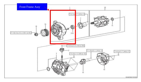
Fig. 7. Alternator Front Frame Assy for component replacement.
