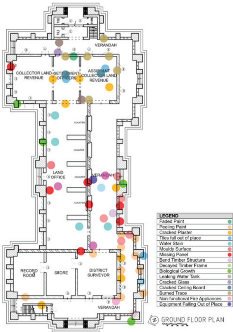
Figure 8. Common Defects in the Ground-floor Area of Case Study 1 Source: Author, 2025
