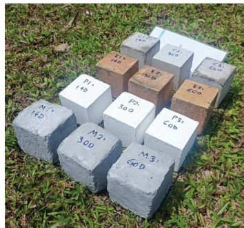
Figure 1. Concrete with Different Repair Material were Exposed to Weather
