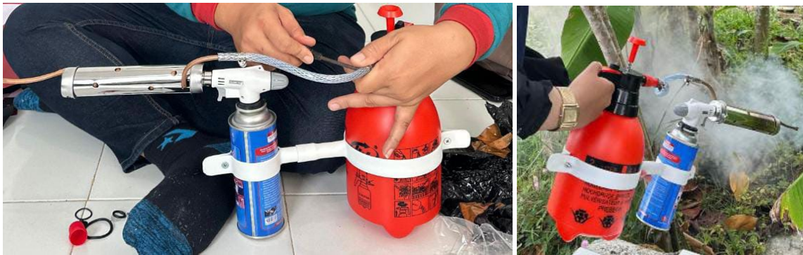
Figure 4. Simple fogging device (low-cost fogging)
