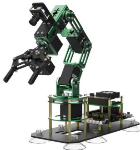
Figure 4. The 6-DOF robotic arm is used for picking up loose fruitlets by implementing deep learning in the inverse kinematic computation for seamless pick-and-place operation.
