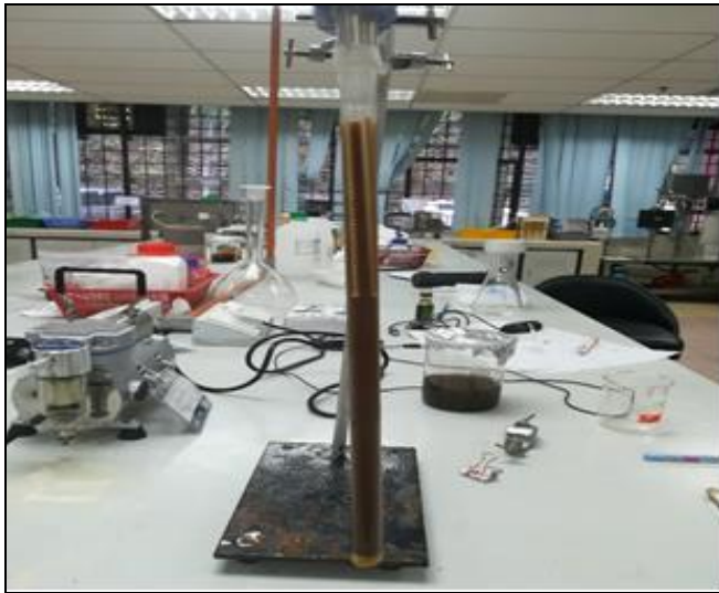
Fig 3 Vacuum suction set up
