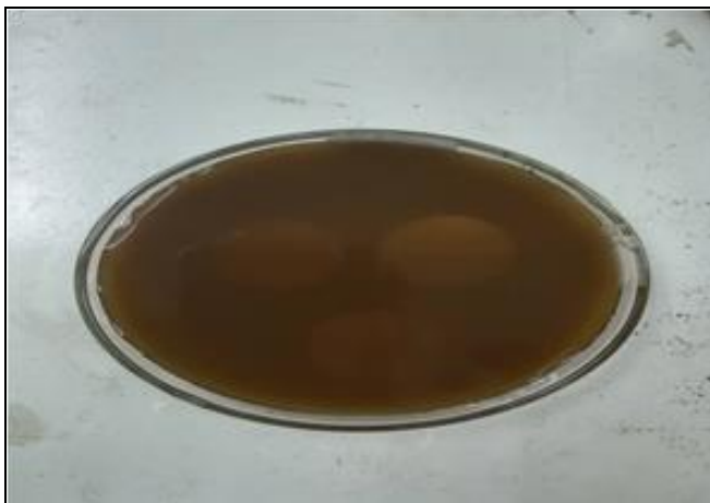
Fig 5 Dip coating method for disc membrane
