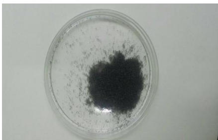
Figure 5c: condition of sand after being coated with chitosan
