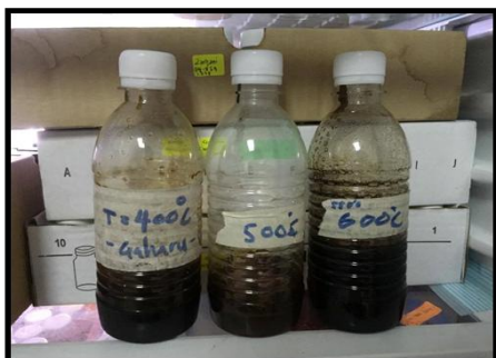
Figure 1: Bio oil produce from pyrolysis of gaharu waste
