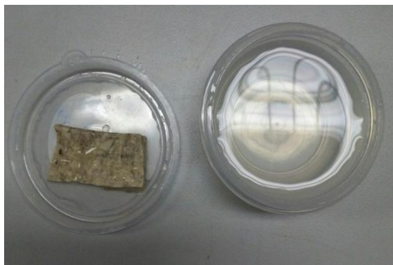
Figure 7 : Natural rubber in diluted toluene exhibit an average Swelling and does not dissolve in the solvent.
