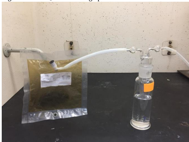
Figure 2: Scrubber bottle in fume chamber.
