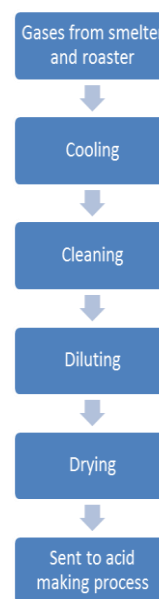
Figure 6: Preparation steps before sent to acid making [16]
